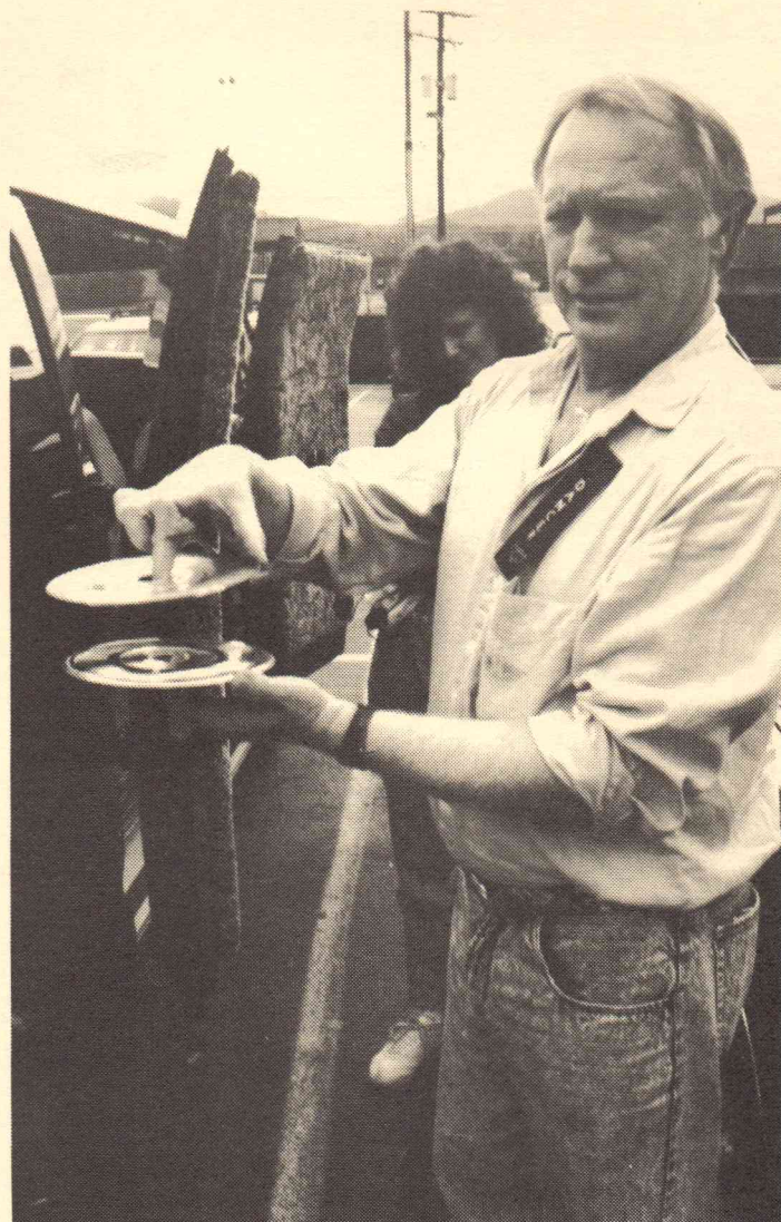
Ralph demonstrates top and bottom half of stamper which presses record and labels, top and bottom.
